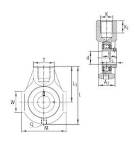
PHEY20 Bearing 2D drawings and 3D CAD models
